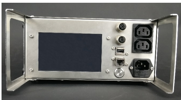
Harmonia in U2 Hephaestus Stainless Steel cabinet. Designed for two independent channels both seen on display. Shown with optional, selectable Electrical-Heating-Blankets.
