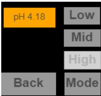
Figure 7 pH calibration screen before Low calibration
