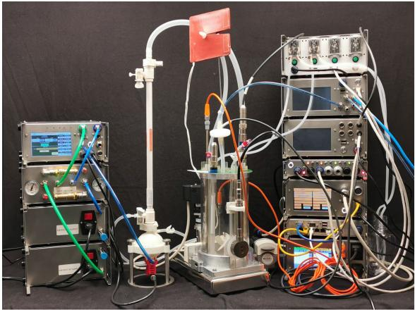
The smaller Clotho-1 is designed for operation of one CellMembra or CellRetention P-SUB's like the one 3.2 litre Vessel Volume seen here. With pressure and vacuum supply to the left side. Here further shown with a complete Process-Control-Systems package on the right side.
