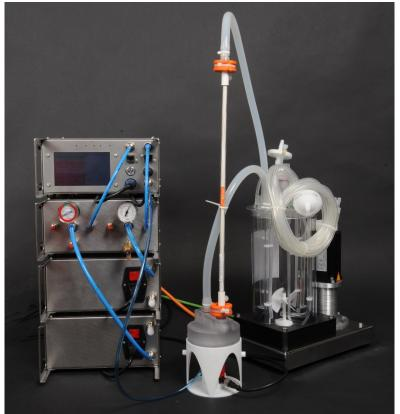
Lachesis-1 is designed for operation of one CellMembra P-SUB's like the one 3,2 litre Vessel Volume seen here. One or more Lachesis-1 may be connected to both Alagonia pumps and Sarpedon reservoir for ease of use.
